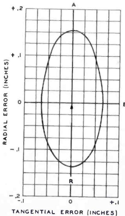
Fig. 19—Computed beam-convergence error pattern plot (32.5 degrees off axis on 12-inch screen).
