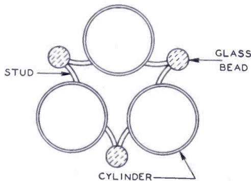
Fig. 4—Three-gun structure having all-beaded support.
