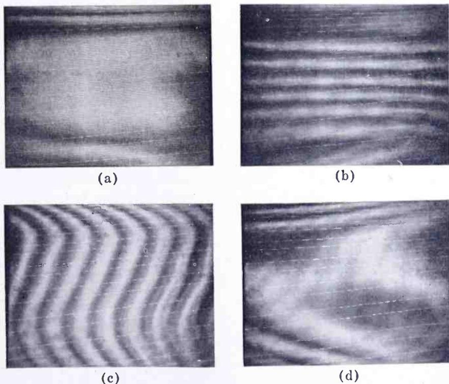
Fig. 2—Typical color fringe patterns of misregistered rasters on line-screen kinescope. (The bright narrow retrace lines should be ignored.) (a) Slight nonlinearity of vertical deflection. Maximum displacement error 0.8 per cent. (b) Vertical size incorrect by 3 per cent. (c) Deflection yoke rotated 1.5 degrees. Sweep linearity same as in (a). (d) Deflection-yoke axis not coincident with electron-gun axis.
