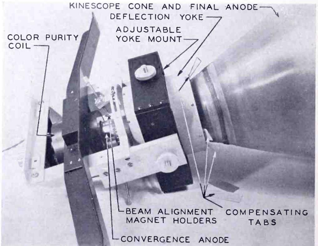
Fig. 22—Assembly of deflection and convergence components on neck of three-gun shadow-mask color kinescope.
