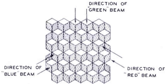
Fig. 8—Cubical-pyramid nonplanar color screen. Sides of cubes facing in different directions are coated with different color phosphors.
