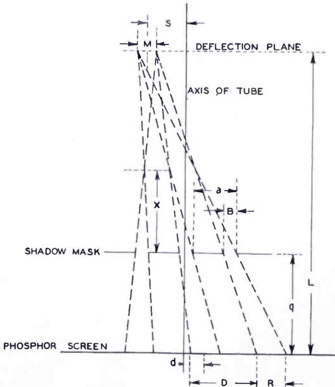
Fig. 5—A plane perpendicular to the shadow mask and passing through a row of holes in the  $y$  direction as defined in Figure 2. The geometry for a source of diameter  $M$  is shown.
