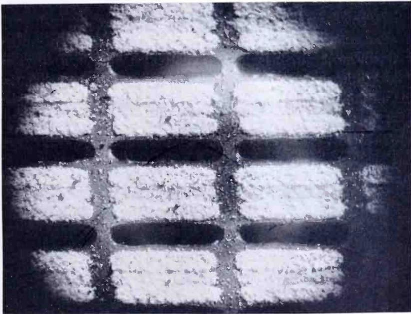
Fig. 8—Photomicrograph of the 3 sets of phosphor strips deposited by settling on the copper aperture plate.
