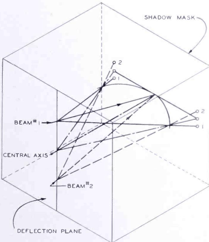
Fig. 16—Deflection normal to plane of beam convergence.
