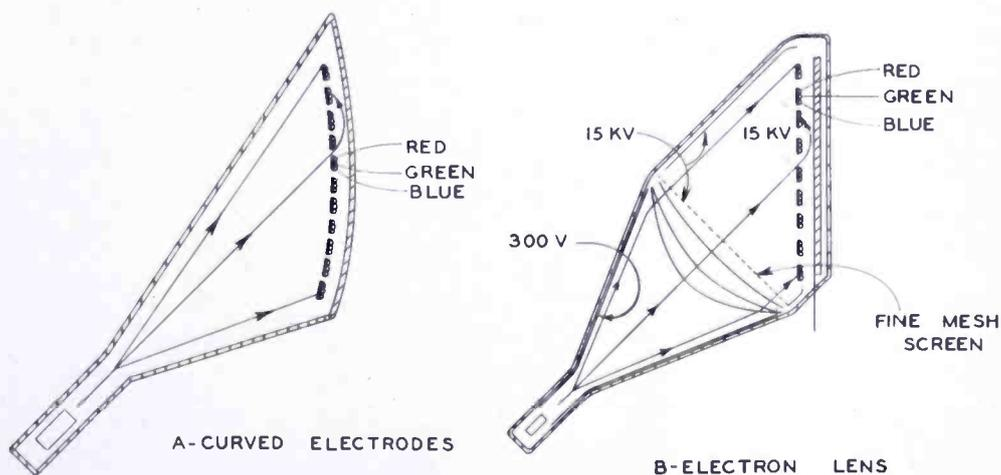
Fig. 4—Two alternative methods of achieving color uniformity by causing the beam to strike the entire screen at 45 degrees. The electrodes in (A) are nonspherical surfaces whose vertical cross section is a spiral and whose horizontal cross section is a circle. The electron lens method in (B) permits plane electrodes to be used and eliminates the need for a “keystoning” correction in the scanning.
