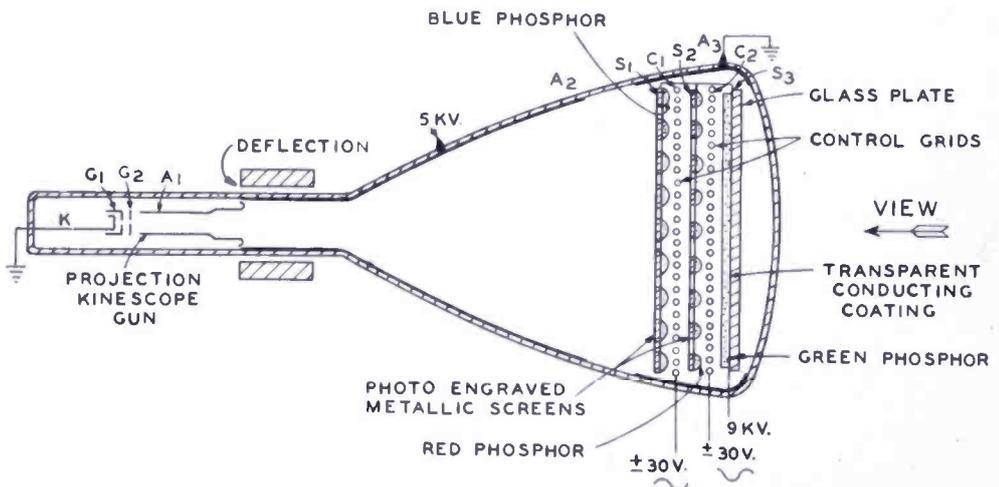
Fig. 4—Three-color single-gun grid-controlled color kinescope.
