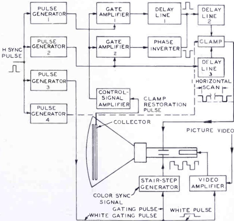
Fig. 8—Aided-tracking circuit employing nonecumulative control.
