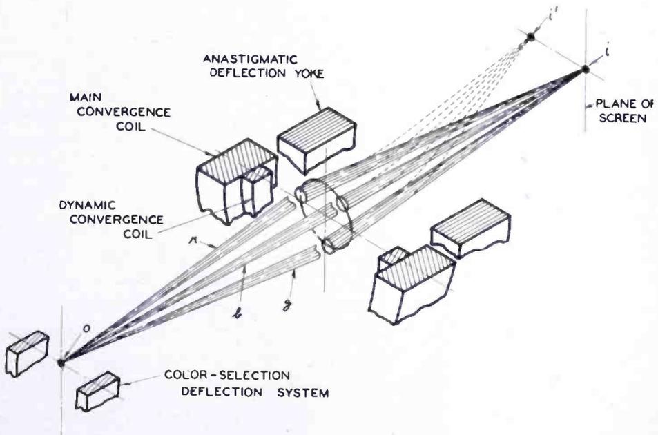
Fig. 1—Electron optics of the one-gun color kinescope.
