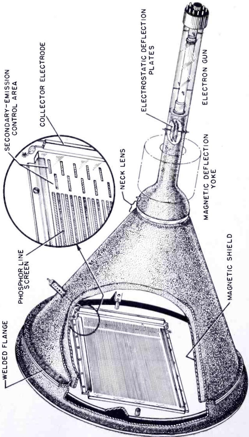
Fig. 1—Sixteen-inch line-screen kinescope.
