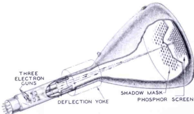
Fig. 3—Experimental shadow-mask color kinescope.
