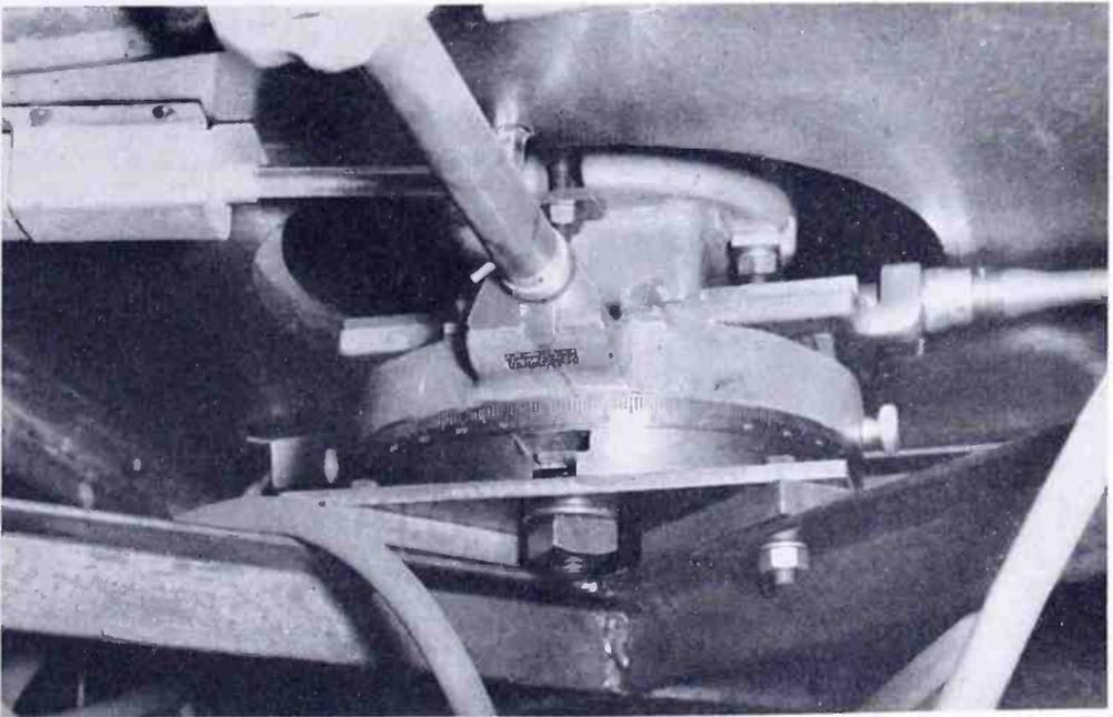
Fig. 2 — Close-up of cross-feed mechanism for positioning phosphor-dot plate on printing table.
