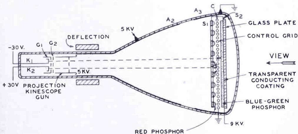
Fig. 3—Two-color two-gun grid-controlled color kinescope.
