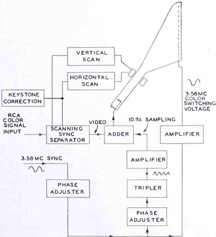
Fig. 11—Block diagram of associated circuits for operating the 45-degree reflection kinescope with the RCA color signal. A 3.58-megacycle sine wave is applied to the reflection plate and a 10.74-megacycle sine wave used for sampling the signal at the gun.
