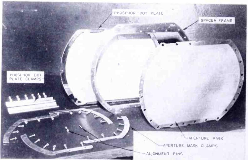
Fig. 3—Viewing-screen assembly—exploded view.
