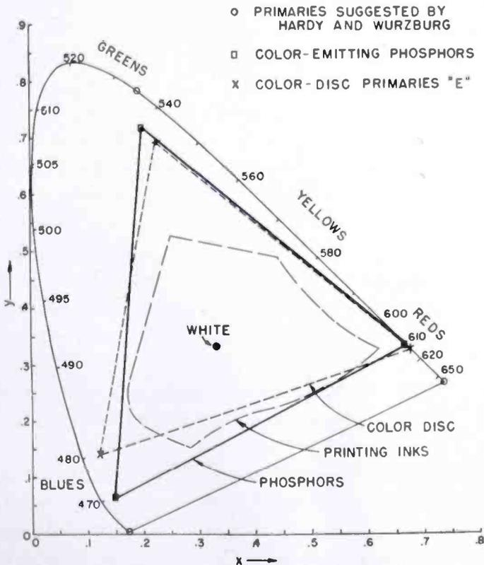
Fig. 1—The I.C.I. color diagram includes all visual colors. The three color primaries achieved by unfiltered phosphors are compared with the color disc and with the idealized primaries of Hardy and Wurzburg. The area possible with modern color printing (according to MacAdam) is shown by the dashed-line figure.
