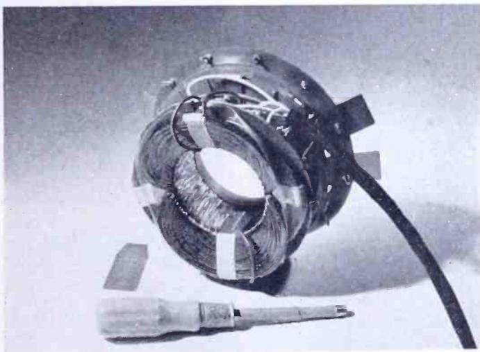
Fig. 14—Rear view of 65-degree deflection yoke of Figure 13, showing tab-clip tightening nuts and mounting of front cover fingers under core clamps.
