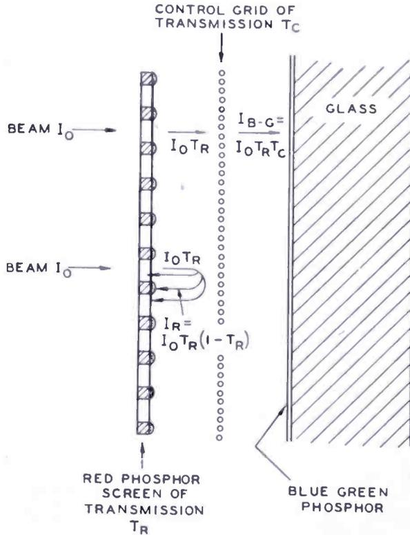
Fig. 7—Currents in two-color kinescope.
