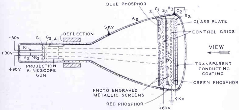
Fig. 5—Three-color three-gun grid-controlled color kinescope.
