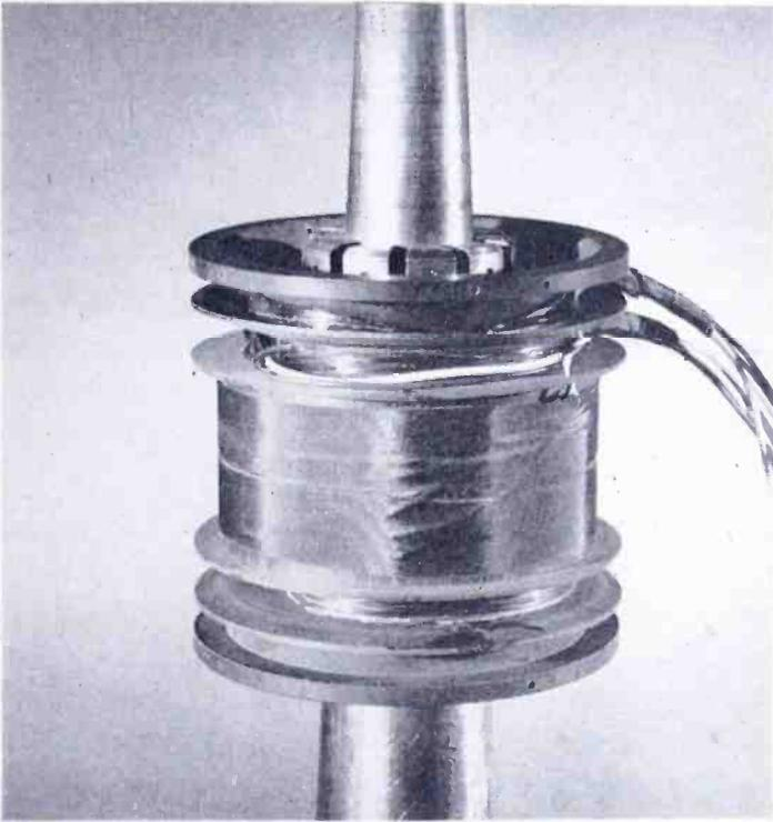
Fig. 4—Coil, core, and spacer assembly of section-wound yoke.
