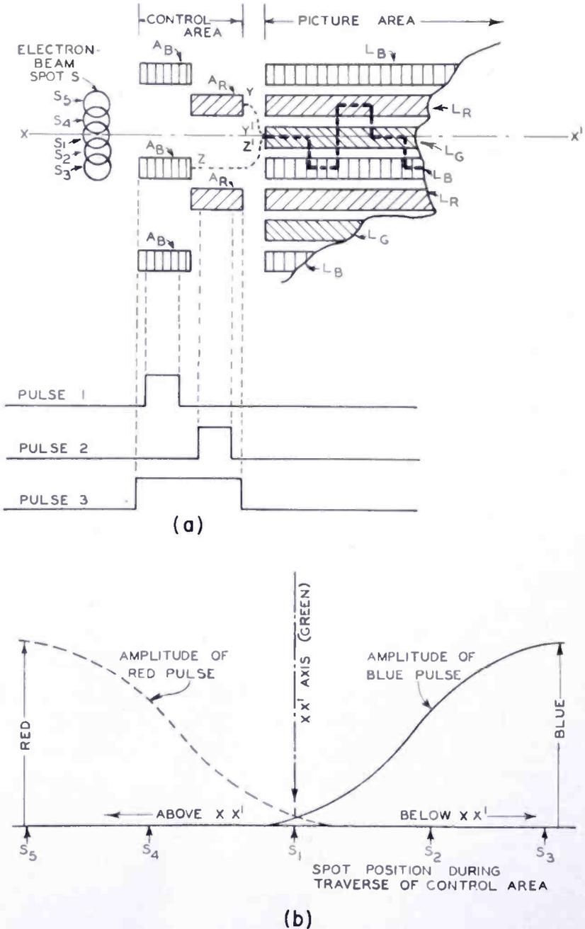
Fig. 7—Control-signal generation process. (a) Beam scanning path in control and picture areas. The times of occurrence of pulses 1, 2, and 3, referred to spot travel, are shown. (b) Amplitude of "red" and "blue" pulses as a function of vertical misregistration of beam in control area. Spot positions  $S_1 \dots S_5$ , shown in (a), are indicated along the abscissa axis.
