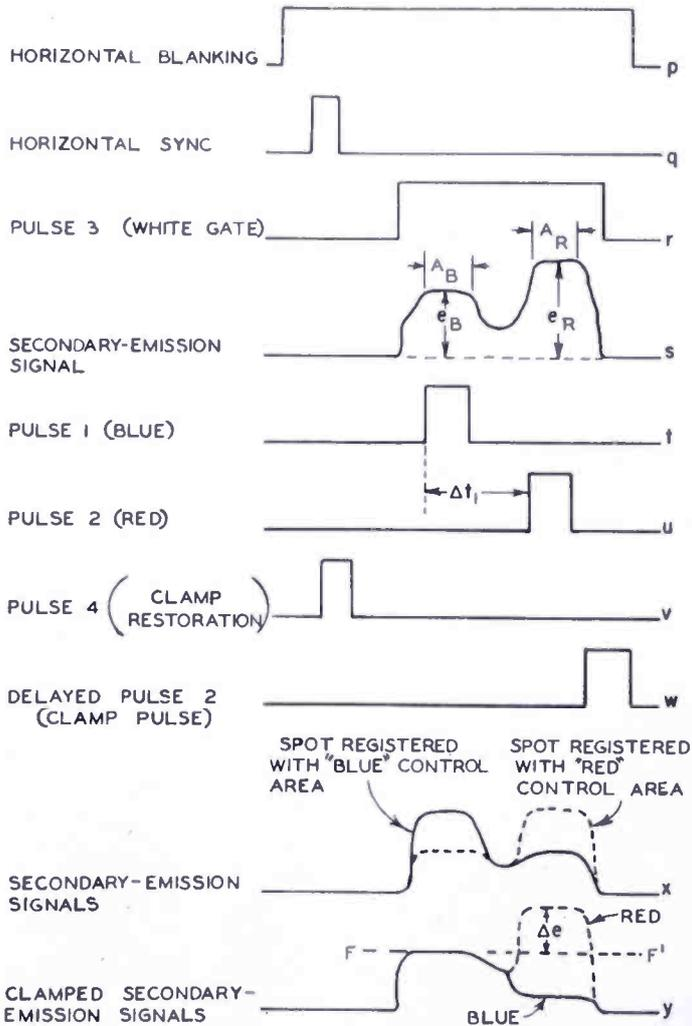
Fig. 9—Diagram of pulses in aided-tracking circuit.
