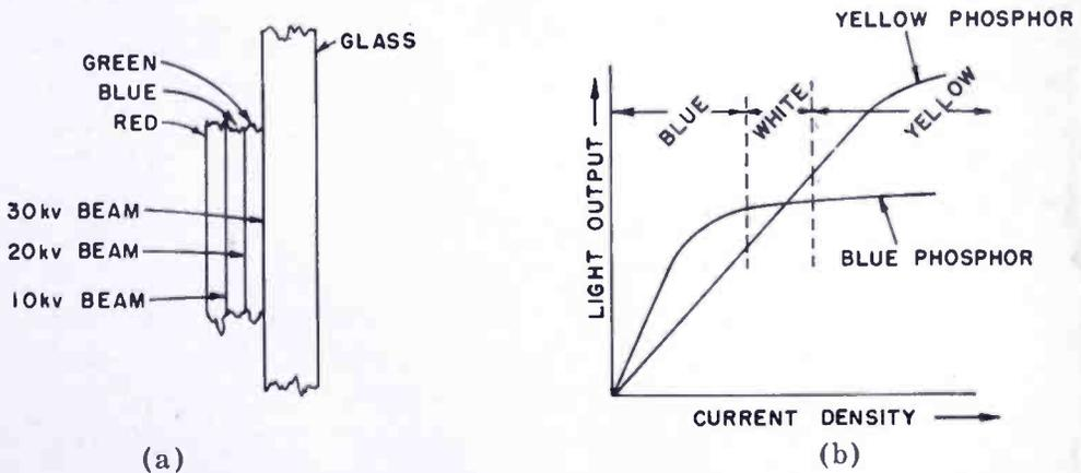
Fig. 4—Multicolor phosphor screen, (a) shows a multiple-layer screen with color depending on beam velocity. (b) shows how saturation in a two-component screen makes color dependent on current density.
