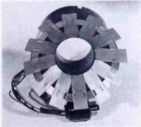
Fig. 9—Array of 12 compensating tabs on section-wound yoke of Figure 5, approximately as used for test of Figures 8c and 8d.
