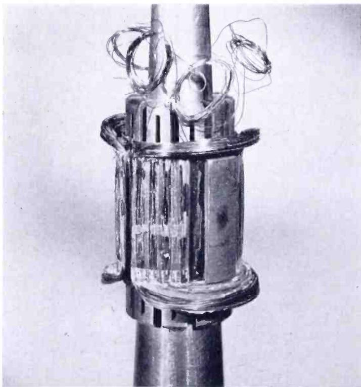
Fig. 3—Horizontal deflection coils and half-cylinder mounts assembled on inner cylinder.
