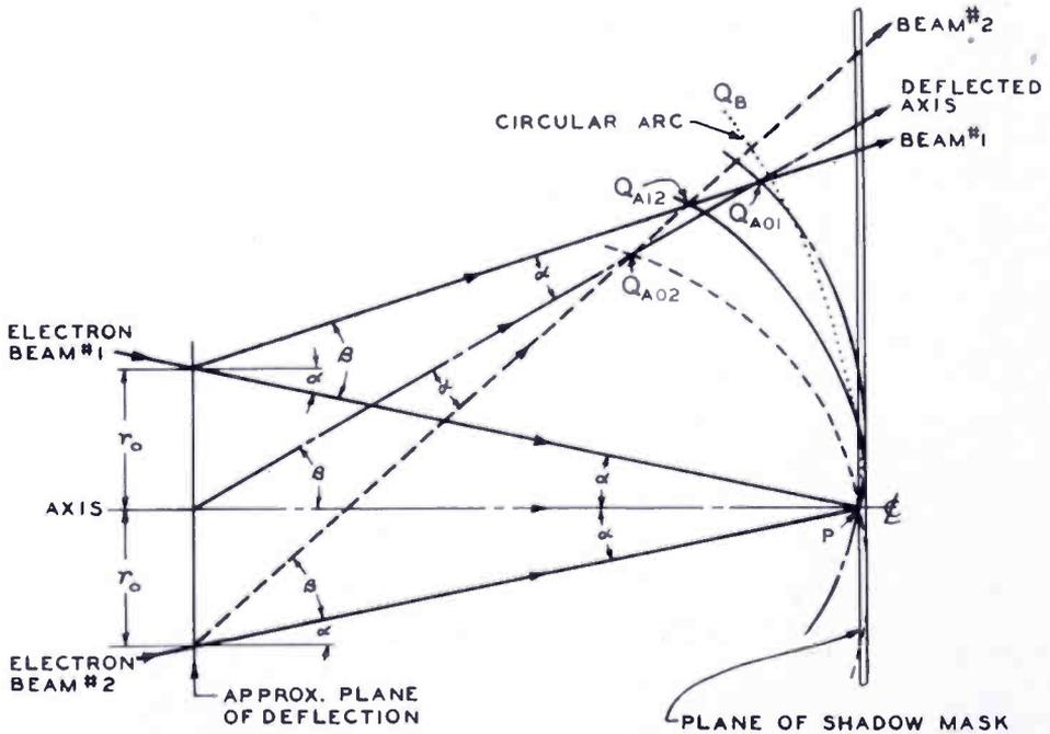
Fig. 17—Simplified geometry of multibeam deflection system.
