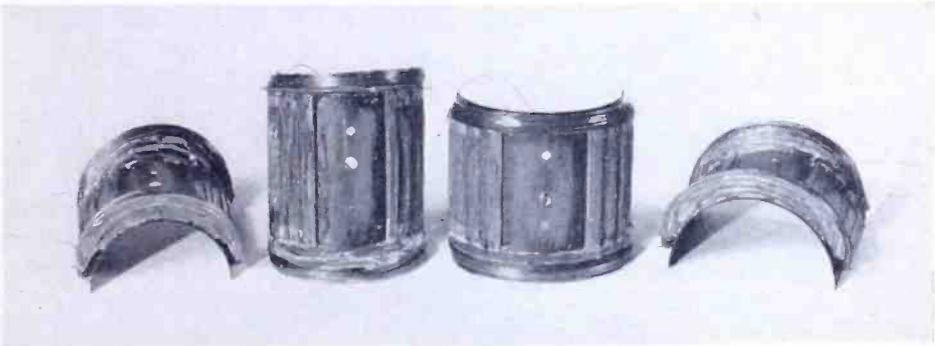
Fig. 2—Section-wound coils on half-cylinder mounts.
