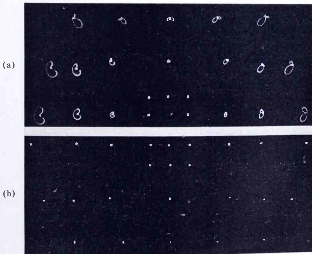
Fig. 7—Spot patterns using an antipincushion yoke, 45-degree maximum deflection angle. (a) Upper half of raster area with large conic beam locus. (b) Lower half of raster area with small electron beam.
