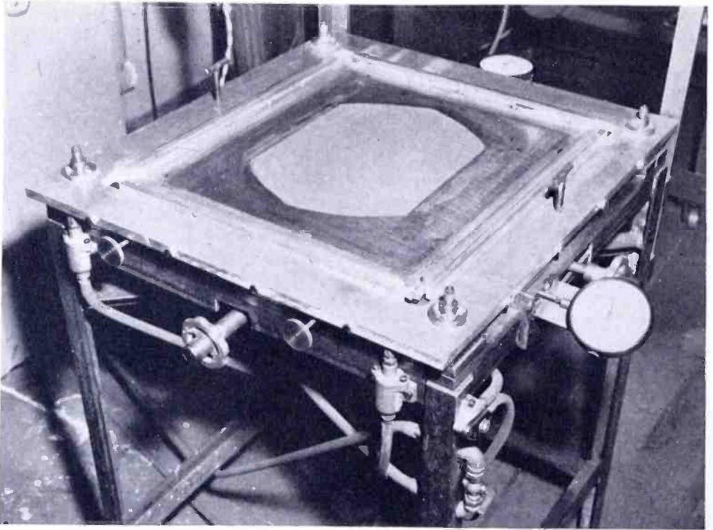
Fig. 1a — Printing table with stencil frame in position.
