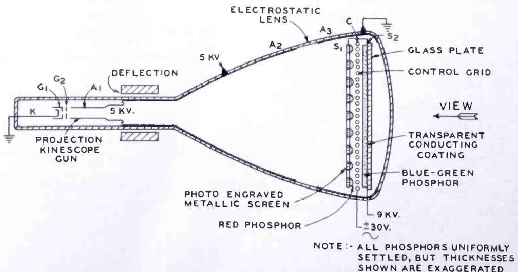
Fig. 2—Two-color single-gun grid-controlled color kinescope.
