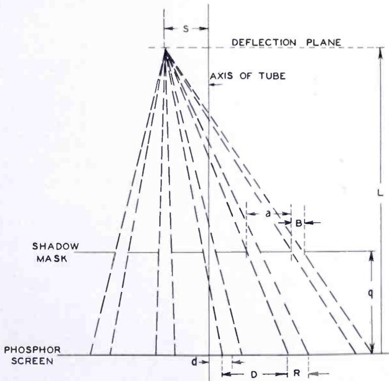
Fig. 4—A plane perpendicular to the shadow mask and passing through a row of holes in the  $y$  direction as defined in Figure 2. The geometry for a point source is shown.
