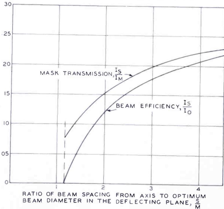
Fig. 7—The efficiency with which the cathode current is utilized and the open area of the mask as a function of  $S/M$  for the optimum values of  $M$  found in Figure 6.
