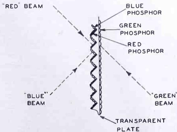
Fig. 7—Baird three-color nonplanar color screen, in principle.
