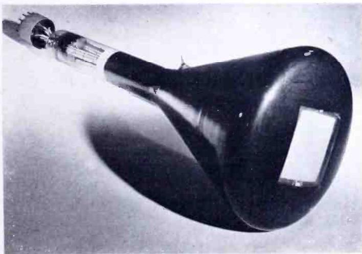
Fig. 8—Experimental shadow-mask color tube containing a test sample of dot screen.
