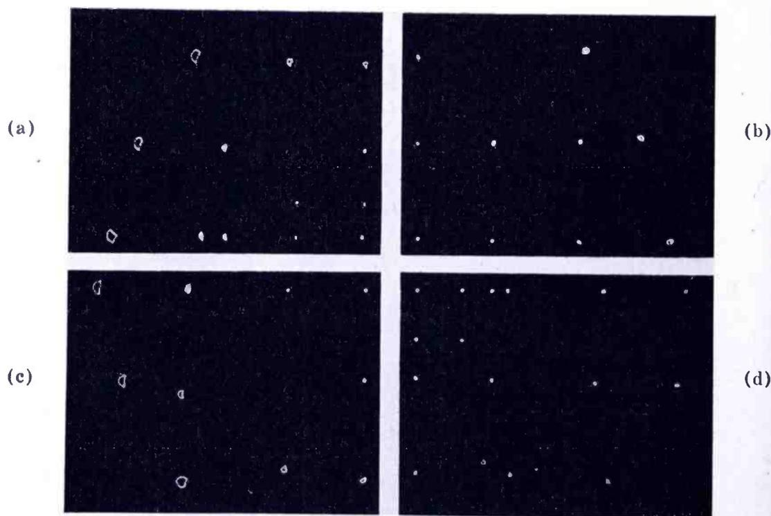
Fig. 8—Spot patterns using section-wound improved convergence yoke of Figure 5, 45-degree maximum deflection angle. (a) Upper left quadrant with convergence correction at center only, no tabs. (b) Upper right quadrant with best convergence correction at each spot position, no tabs. (c) Lower left quadrant, convergence correction at center only, 12 compensating tabs adjusted. (d) Lower right quadrant, with best convergence correction at each position, 12 tabs adjusted (final result).
