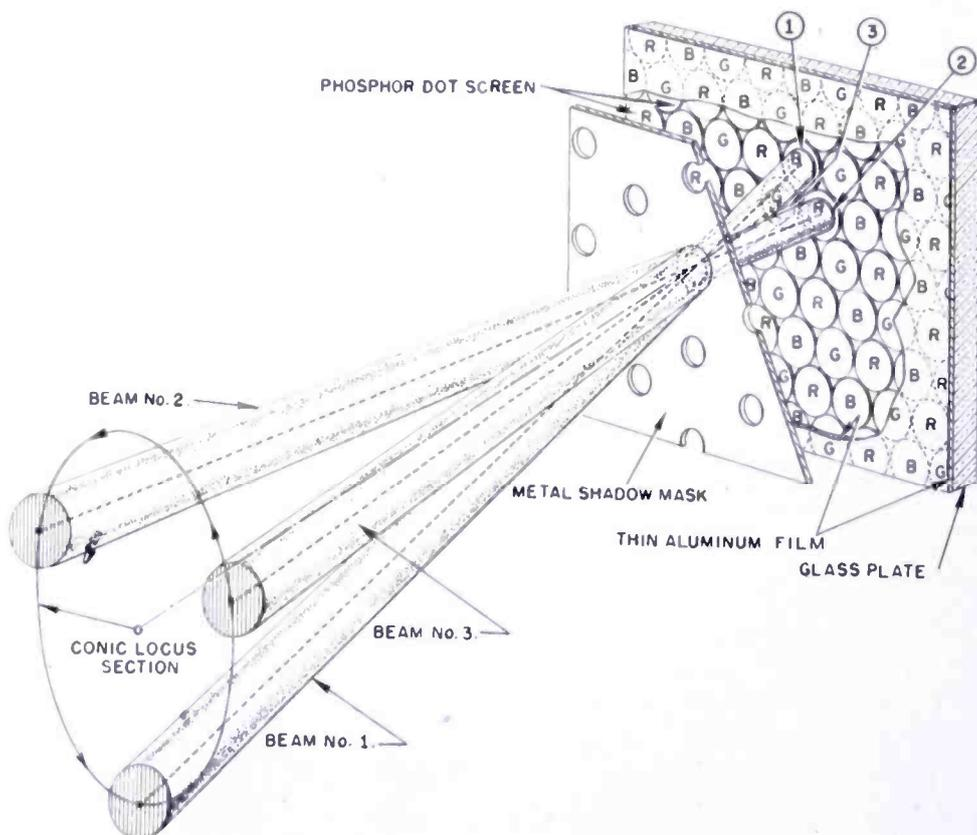
Fig. 1—Electron beams on conic locus.
