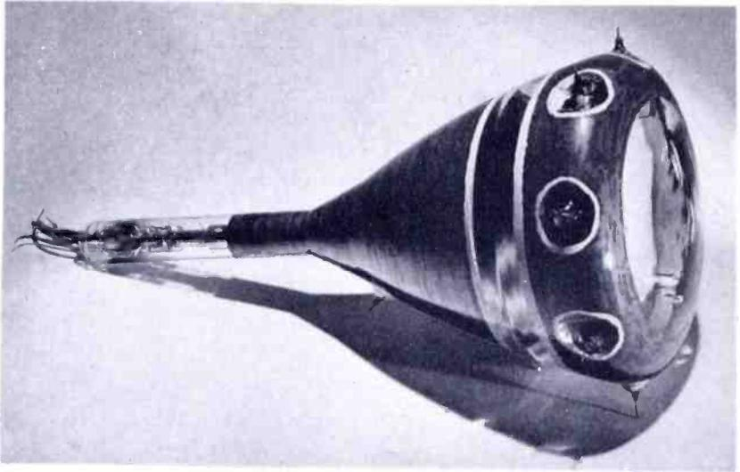
Fig. 1—Experimental grid-controlled color kinescope.
