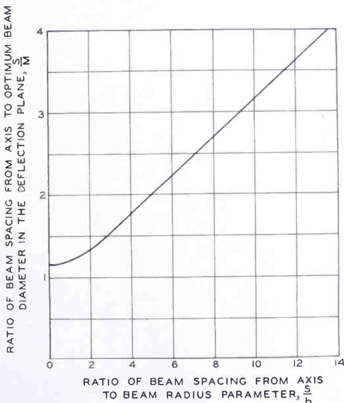
Fig. 6—Plot of the relation between  $b$ ,  $S$ , and the corresponding optimum value of  $M$ .  $S$  is the distance between the axis and the center of each beam in the center-of-deflection plane,  $M$  is the diameter of the electron beam in the center-of-deflection plane, and  $b$  is the radius of the beam in that plane at which the current density in the beam has reduced to  $1/e$  of its maximum value.
