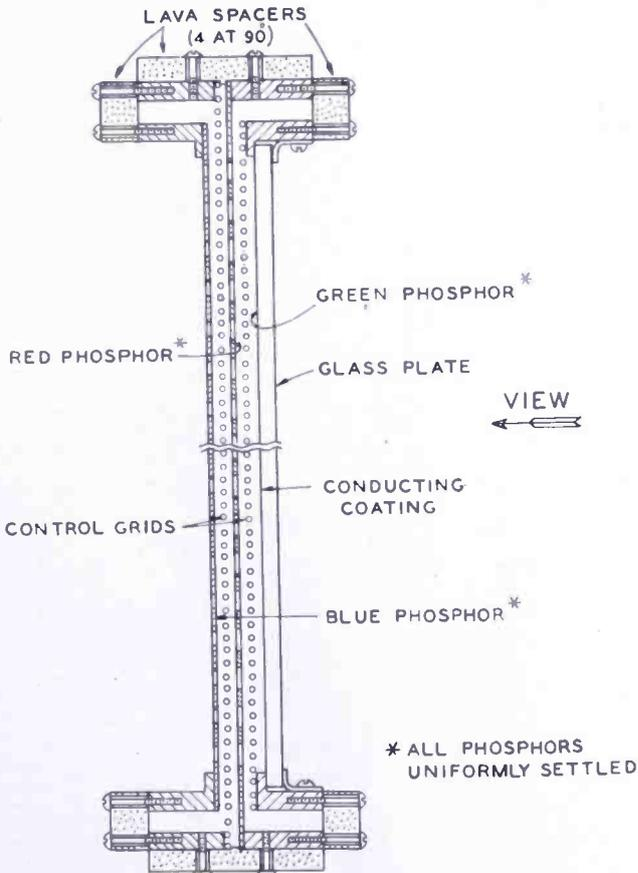
Fig. 6—Screen assembly, three-color grid-controlled color kinescope.
