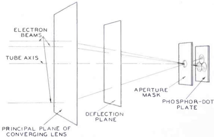
Fig. 2—Diagram illustrating three-beam convergence.
