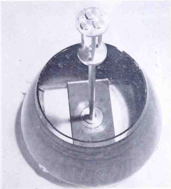
Fig. 10—Jig for locating the electron guns with respect to the phosphor-screen assembly in an experimental shadow-mask color kinescope.
