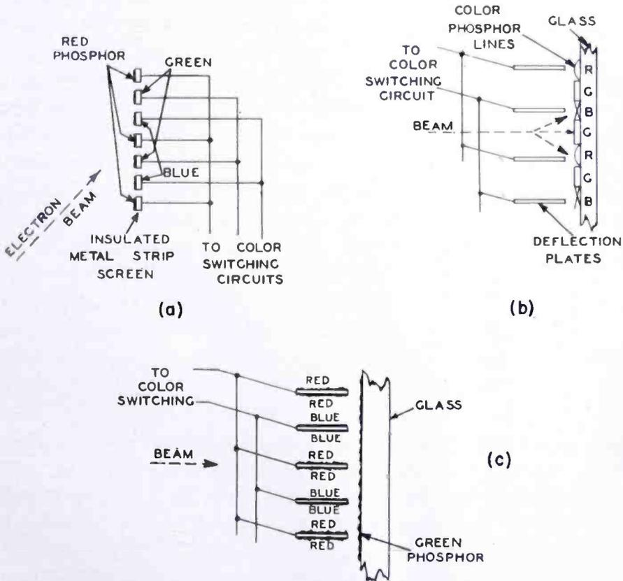
Fig. 5—Beam control at phosphor screen for changing color. (a) Simple line-screen color switching. (b) Deflection switching of colors with line screen. (c) Deflection switching without requiring registry.
