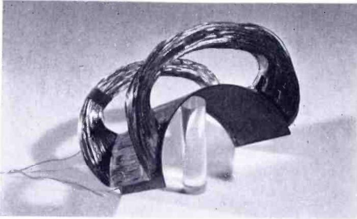
Fig. 10—Sectional-wound yoke coil with elevated turn-ends.
