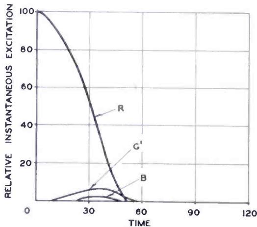
Fig. 10—Time variation of relative instantaneous excitation of each color due to single primary-color signal.
