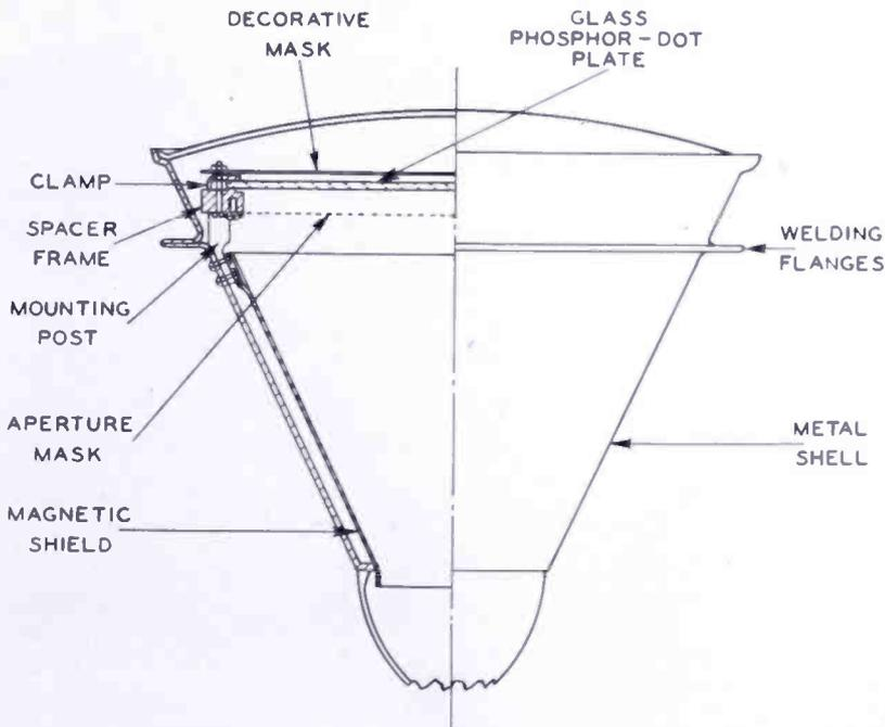
Fig. 2—Cross section of envelope.
