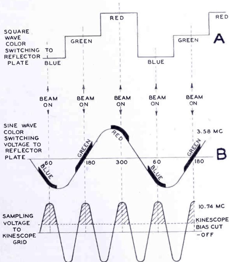
Fig. 10—Wave forms of the color-switching voltage which may be applied to the reflector plate. For low-speed switching the step wave shown in A would be preferable. For high-speed switching at megacycle frequencies the sine wave shown in B was entirely suitable. Beam blanking at three times the switching frequency was used to give the required color sequence.
