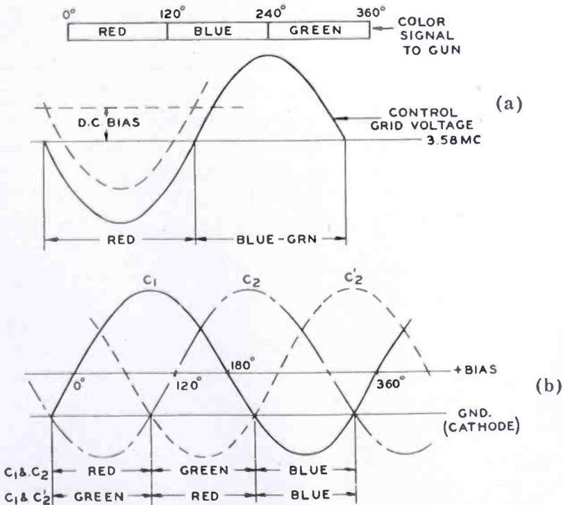
Fig. 8—Sine-wave switching of grid-controlled kinescope: (a) two-color; (b) three color.
