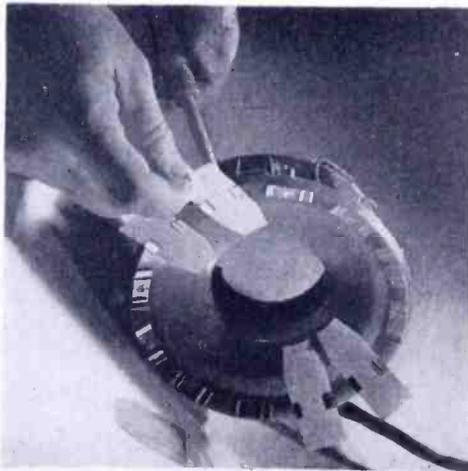
Fig. 13—Front view of 65-degree multibeam deflection yoke adapted for machine winding and die forming. Four compensating tabs are shown in place on moulded polyethylene mounting cover.
