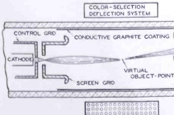
Fig. 6—Developmental simplified short electron gun.
