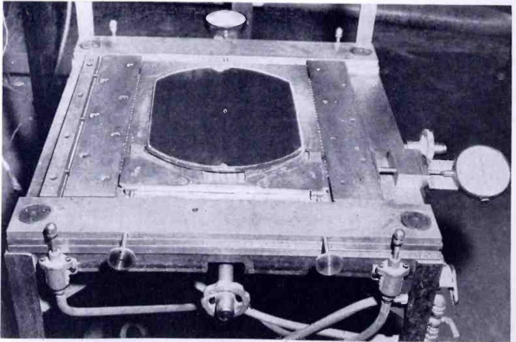
Fig. 1b — Printing table with stencil frame removed. Two air pistons are visible in front.
